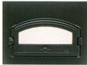
#0214 mat black, gasketed, with frame (600 x 443), hinged right or left 410 x 230 x 180 mm (16 1/8" x 9 1/16" x 7 1/8") weight 16 kg.
